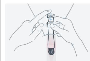
Insert Pippa Grip the Spring holder at the rim, between the forefinger and thumb.
